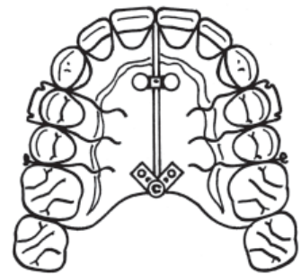
Fan Type Used when only anteriors need to be expanded. Can be reversed to only expand posterior segments.
